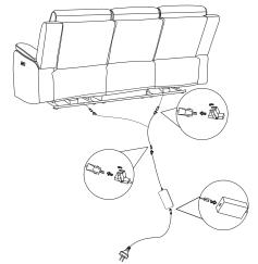
Safety Note: Transformer and cables are not to be placed under or within the recliner structure.
